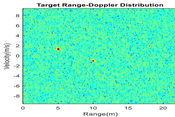
**Figure 9** Target Range-Doppler Distribution.
