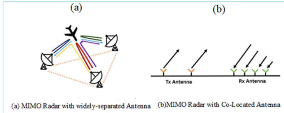
**Figure 4** (a)MIMO Radar with widely-separated Antenna and (b)MIMO Radar with Co-Located Antenna.
