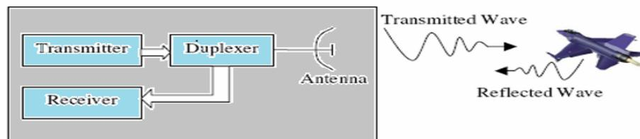
**Figure 1** Simple monostatic radar configuration
