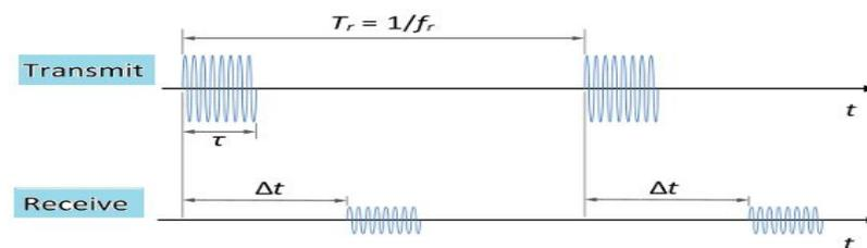
**Figure 2** Signal waveforms in pulse-modulated radar. The delay and received power are related to the range of objects.
