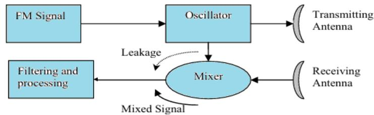
**Figure 3** Block diagram of a simple FM-CW radar.
